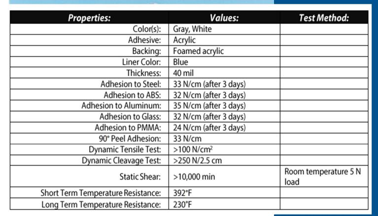
Carter's Structural Stiffener Tape is a 40 mil high bond tape, designed to adhere to our Integrated Stiffener with a perfect width of 1.25" for full coverage.
